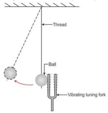
It is noticed that as the arm of the vibrating fork is brought close to the ball, it jumps back and forth and sound of the vibrating tuning fork is heard. When its arm stop vibrating, the ball becomes stationary and no sound is heard.
