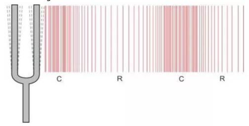
Compressions are the regions of high density where the particles of the medium come very close to each other and rarefactions are the regions of low density where the particles of the medium move away from each other.
